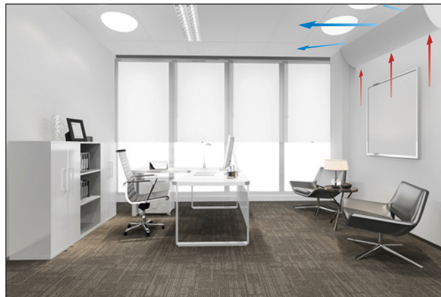
Picture 46. Plafond XD-FC with Cover type Badge. Installation principle "wall/beam".
