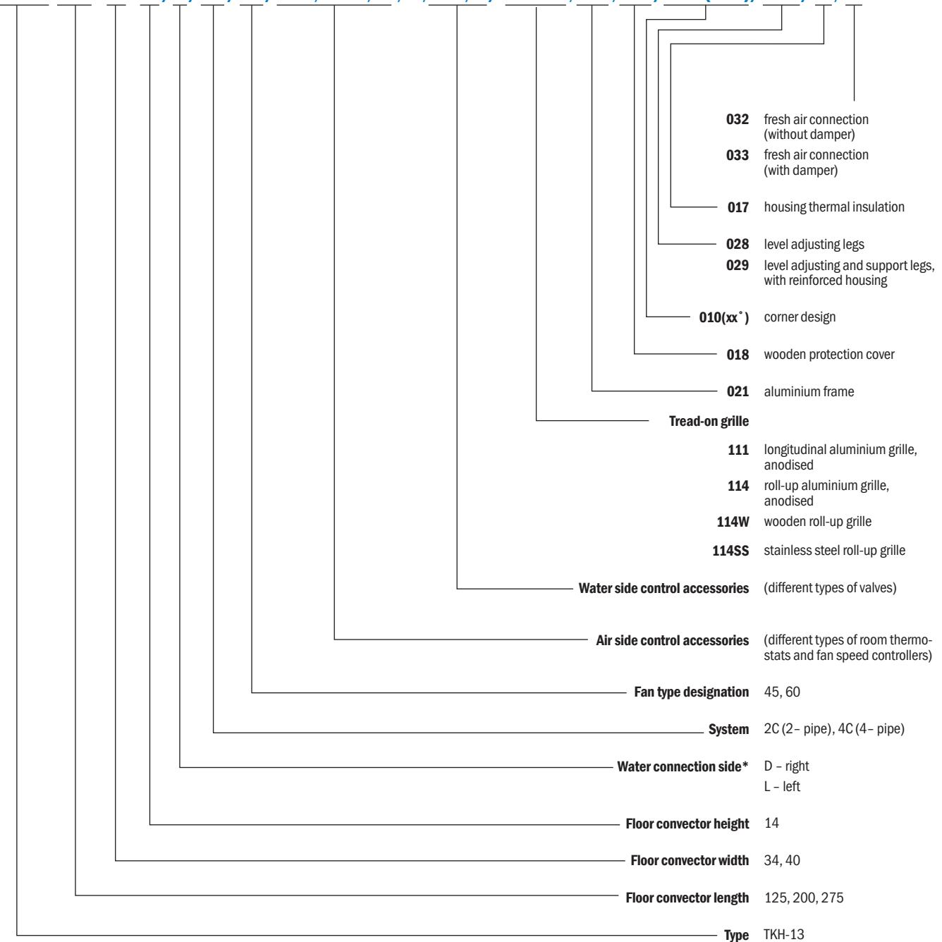
\*Designation L (left) and D (right) indicate the side water connections, whereby it is necessary to look at the convector from the room towards the window.
